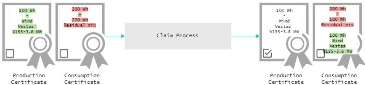
Figure 14 The final validation of consumption and production certificate claims, stamps the consumption certificate with the attributes of the production certificate.
