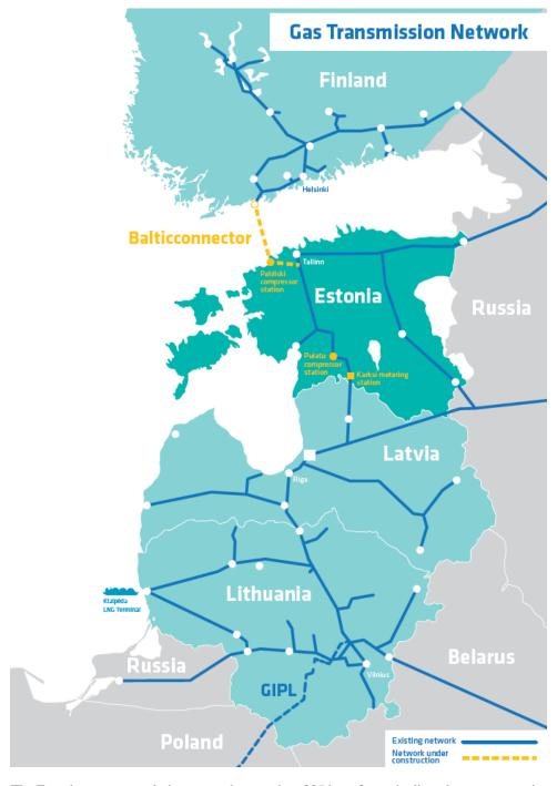
The Estonian gas transmission network comprises 885 km of gas pipeline, three gas-metering stations and 36 gas distribution stations. The Gas Network also connects to gas transmission networks in Latvia and Russia, as shown in the diagram of the Gas Network above.
