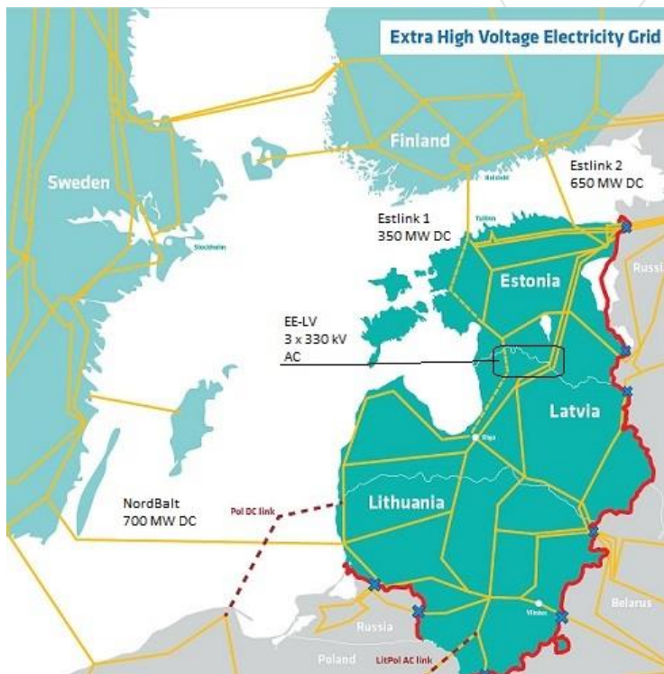
Drawing 5.1 – Baltic main grid with connections
